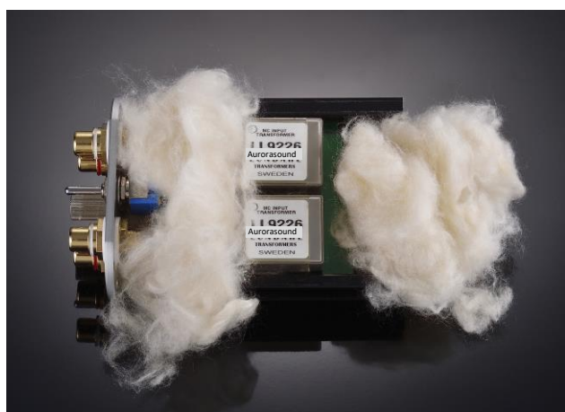
Filled with pure cotton, to reduce the influence of external vibrations
