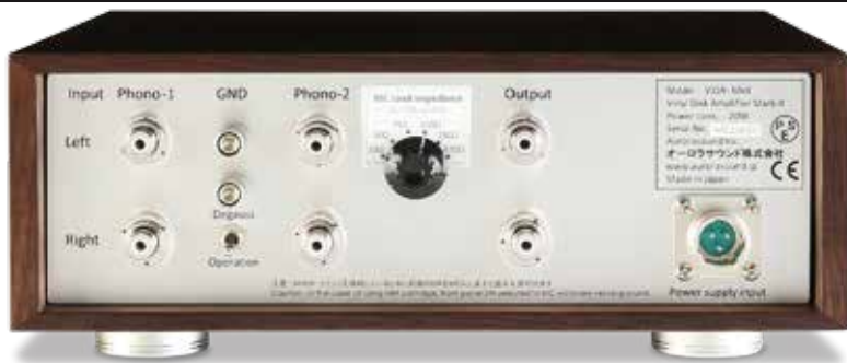
ABOVE: The MkII still offers two front-switched MM/MC phono inputs, but brings the degauss function to the rear. Variable 30-470ohm (low) MC loading option is extra
