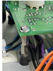
Seismic isolation for vacuum tubes protection
