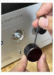
5 つまみを入れてLレンチでビスを締めます Place the wood knob and fix the screw by L-wrench
